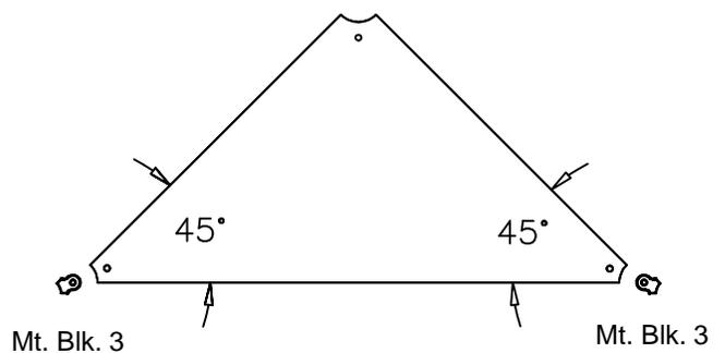
Mounting Block 3 is used ONLY on the 45° corners of this deck, 2 Pl.
